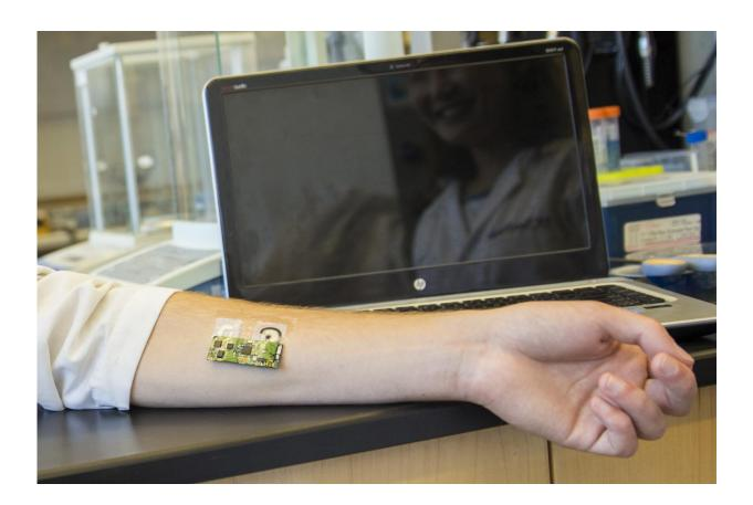
This flexible wearable sensor can be worn on the arm to detect alcohol level. Credit: UC San Diego
