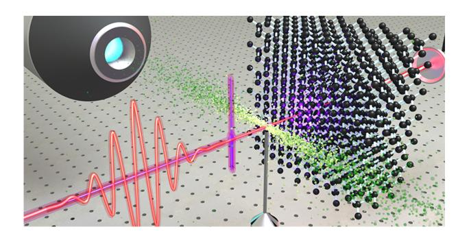
A short laser pulse travels through a diamond (black spheres) and excites electrons inside it. The strength of the excitation is measured using an attosecond ultraviolet pulse (violet). Credit: Matteo Lucchini, ETH Zurich
