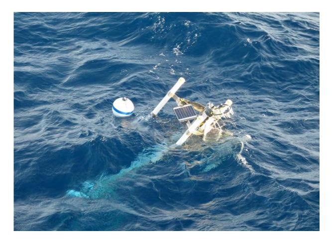
A Son-O-Mermaid instrument in the water. The research team deployed and retrieved the buoys several times to test that everything was working and to identify remaining kinks. Now the task ahead is to construct a robust new generation of Son-O-Mermaid instruments to add to the growing number of earthquake recorders in the oceans. With each new instrument deployed, Simons and colleagues will help fill in the picture of our planet's interior. Credit: Princeton University
