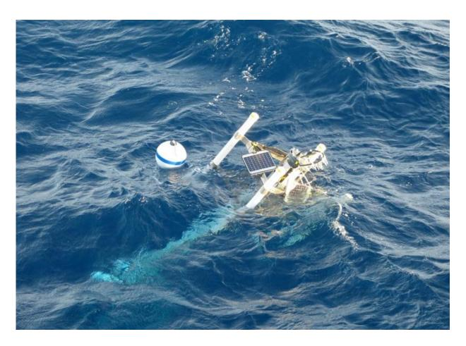
A Son-O-Mermaid instrument in the water. The research team deployed and retrieved the buoys several times to test that everything was working and to identify remaining kinks. Now the task ahead is to construct a robust new generation of Son-O-Mermaid instruments to add to the growing number of earthquake recorders in the oceans. With each new instrument deployed, Simons and colleagues will help fill in the picture of our planet's interior. Credit: Princeton University
