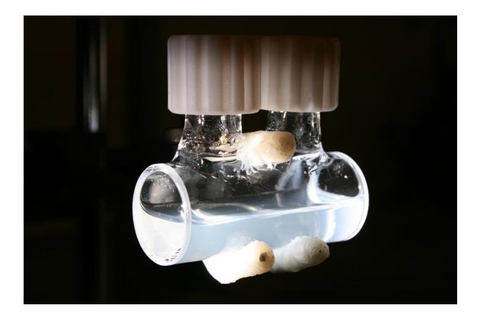
The photochemical reactor used to investigate the photochemistry at the air-sea interface. Credit: Monica Passananti
