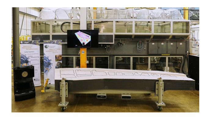
A 3-D printed trim tool developed by ORNL and Boeing to be used in building Boeing's 777X passenger jet has received the title of largest solid 3-D printed item by GUINNESS WORLD RECORDS. Credit: ORNL
