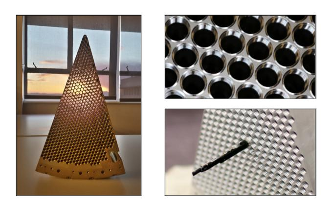
The first "petal" machined for the Dark Energy Spectroscopic Instrument (DESI) is shown in these photos. Ten of these petals, which together will hold 5,000 robots (like the one in the lower right photo) -- each pointing a thin fiber-optic cable at separate sky objects -- will be installed in DESI. Credit: Joe Silber/Berkeley Lab
