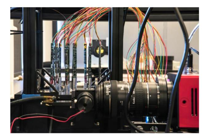
This is a view of the ProtoDESI setup during assembly at Berkeley Lab, with the underside of the robotic fiber-positioners visible at left. ProtoDESI is now installed at the 4-meter Mayall Telescope at Kitt Peak National Observatory near Tucson, Ariz. Credit: Paul Mueller/Berkeley Lab
