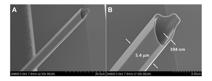
These potassium diphosphate (KDP) crystals, which self-assemble in solution as hollow hexagonal rods, could find use in laser technology, particularly for fiber-optic communications. The scanning-electron image at right shows a crystal at higher resolution with scale added. Credit: L. Deng / NIST
