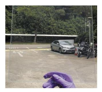
A\*STAR researchers have developed a window coating that lets visible light through while blocking near-infrared radiation. Credit: A\*STAR Singapore Institute of Manufacturing and Technology
