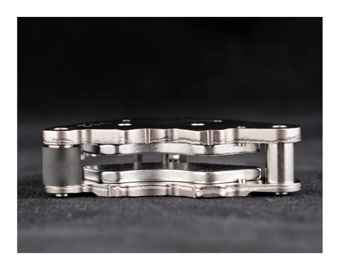
Rare earth magnet assembly was recovered from a used hard drive. Credit: ORNL
