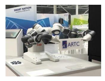
YuMi from ABB is a dual arm collaborative robot that can assemble, pick and sort through small components. Credit: A\*STAR Advanced Remanufacturing and Technology Centre
