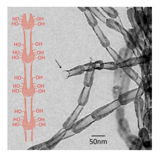
The black arrow indicates the end of the opening of carbon nanopot. A structural schematic of the carbon nanopot showing hydroxyl groups bonded to the edges of the graphene layers near the closed end of the nanopot is also indicated (not to scale). Credit: *Journal of Materials Research*, 31((1): 117-126, 14-Jan-2016, doi:10.1557/jmr.2015.389.Copyright: Materials Research Society
