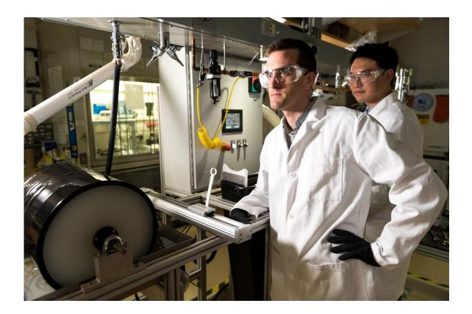
Georgia Tech Assistant Professor Ryan Lively (left) and Postdoctoral Fellow Dong-Yeun Koh monitor the spinning process used to produce the polymeric fibers that are converted for use in the carbon membranes used for separating alkyl aromatic chemicals. Credit: Rob Felt, Georgia Tech
