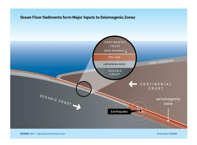
Schematic diagram of a subduction zone with sediments structure. Credit: C. Kersten GEOMAR
