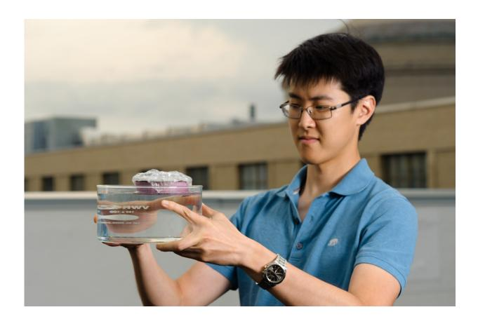
MIT graduate student George Ni holds a bubble-wrapped, sponge-like device that soaks up natural sunlight and heats water to boiling temperatures, generating steam through its pores. Credit: Massachusetts Institute of Technology
