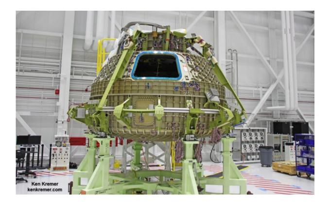
Hull of the Boeing CST-100 Starliner Structural Test Article (STA)- the first Starliner to be built in the company's modernized Commercial Crew and Cargo Processing Facility high bay at NASA's Kennedy Space Center in Florida. Credit: Ken Kremer/kenkremer.com
