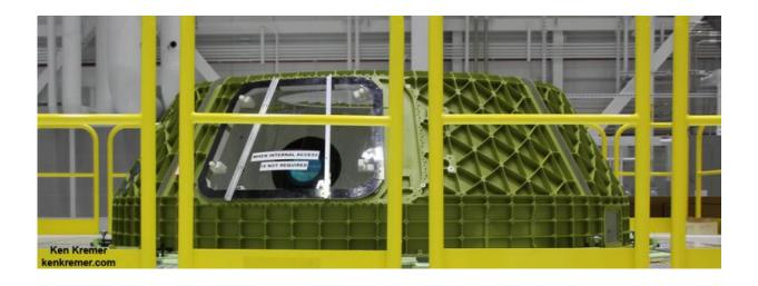
The honeycombed upper dome of a Boeing Starliner spacecraft on a work stand inside the company's Commercial Crew and Cargo Processing Facility at NASA's Kennedy Space Center in Florida. The upper dome is part of Spacecraft 1, the first flightworthy Starliner being developed in partnership with NASA's Commercial Crew Program. Credit: Ken Kremer/kenkremer.com
