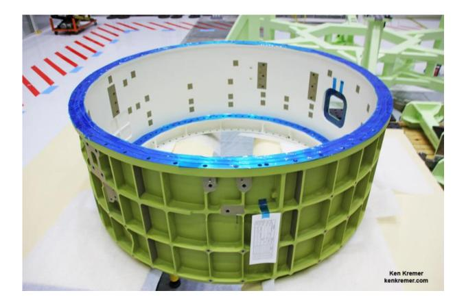
Overhead view of the docking hatch for the Boeing Starliner Spacecraft 1 assembly which technicians will soon join to the upper dome in the firm's Commercial Crew and Cargo Processing Facility high bay at NASA's Kennedy Space Center in Florida. Credit: Ken Kremer/kenkremer.com
