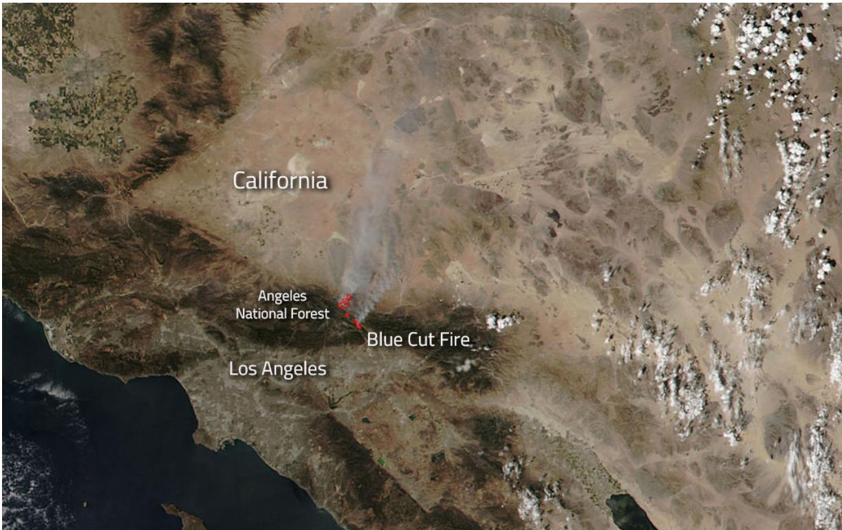
NASA's Suomi NPP satellite collected this natural-color image using the VIIRS (Visible Infrared Imaging Radiometer Suite) instrument on August 17, 2016. Actively burning areas, detected by thermal bands, are outlined in red. Credit: NASA image courtesy Jeff Schmaltz LANCE/EOSDIS MODIS Rapid Response Team, GSFC.
