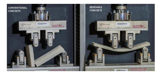
Conventional Concrete vs Bendable Concrete developed at NTU. Credit: Nanyang Technological University
