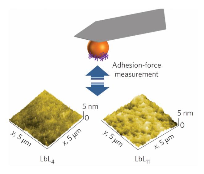
Force measurements on reference material. Credit: University of Twente
