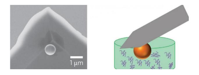
Modified AFM cantilever to which protein molecules will attach. Credit: University of Twente
