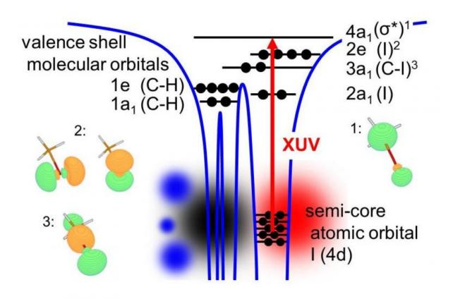
Fig. 1: Fig.1: XUV absorption from the core shell to vacancies in the valence shell are element specific and sensitive to the local chemical environment around the reporter atom. Credit: Forschungsverbund Berlin e.V. (FVB)
