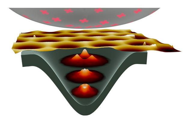
The charged tip of a scanning tunneling microscope and an additional magnetic field lead to localized stable electron states in graphene. Credit: Nils Freitag, RWTH Aachen
