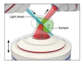
By adding a third objective lens, researchers were able to capture previously neglected fluorescence, improving image resolution in three dimensions. The schematic on the right shows the new approach as applied to a type of light-sheet microscopy. Credit: Yicong Wu, National Institute of Biomedical Imaging and Bioengineering
