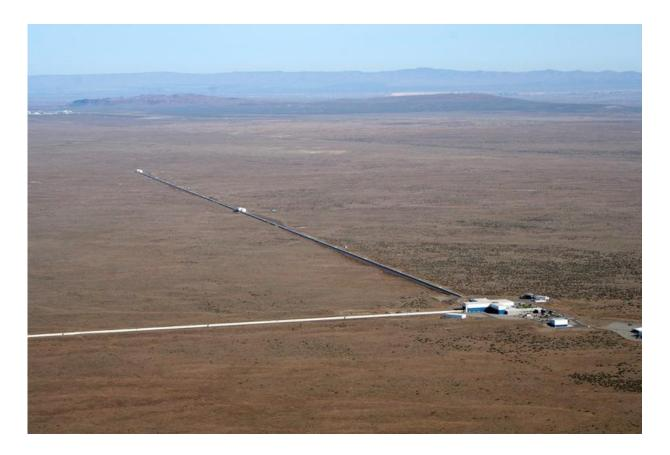
An aerial view of the Advanced LIGO site in Hanford, Washington, shows the Lshaped experiment. Each arm is 2.5 miles long. Credit: SLAC National Accelerator Laboratory
