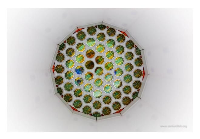
The LUX dark matter detector is surrounded by light sensors that can detect the emission of just a single photon. Those sensors are designed to capture the tiny flash of light emitted if a dark matter particle were to interact with the detector's xenon target material. Credit: Matt Kapust/ Sanford Underground Research Facility
