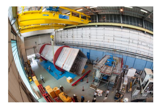
The ICARUS cryostat is being rotated so that aluminium welding can always be done in a flat position. Credit: M.Brice/CERN
