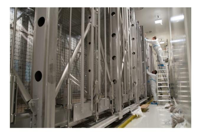
One of the ICARUS time projection chambers being refurbished at CERN in a clean room. Credit: Max Brice/CERN
