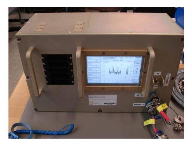
The new European Crew Personal Active Dosimeter – EuCPAD – comprises wearable units plus this storage device for battery charging and data transfer – similar in purpose to a smartphone charging station, if much more sophisticated. A storage device has been launched to ISS on 18 July 2016. Credit: ESA
