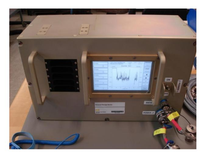
The new European Crew Personal Active Dosimeter – EuCPAD – comprises wearable units plus this storage device for battery charging and data transfer – similar in purpose to a smartphone charging station, if much more sophisticated. A storage device has been launched to ISS on 18 July 2016. Credit: ESA
