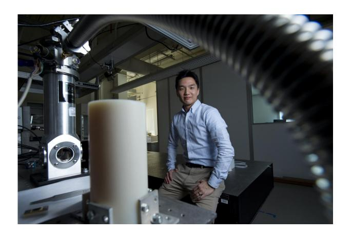
Jaeho Lee's nanomaterials lab at UCI features a customized vacuum chamber that allows samples to be heated to enormous temperatures. By doing so, he can determine whether the substances have suitable thermoelectric properties. Credit: Steve Zylius / UCI
