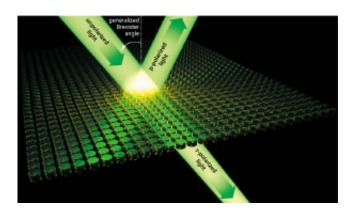
A periodic array of nanodisks in a silicon surface can generate two kinds of polarized light from any angle. Credit: A\*STAR Data Storage Institute
