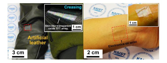
Ultrathin, flexible, and transparent oxide thin-film transistors attached to a jumper sleeve and human skin. Credit: KAIST
