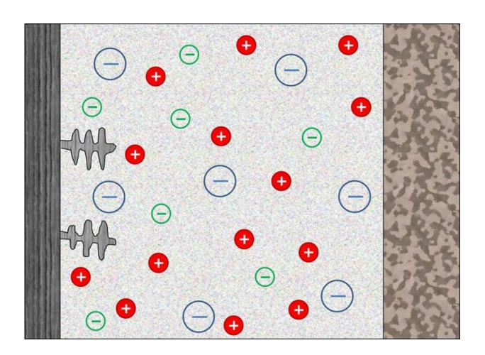
An illustration of the electrolyte inside a rechargeable battery, with the large blue spheres representing the immobile anions tethered to a solid matrix. The small red and green spheres represent the positive and negative ions, respectively; at left are dendrites, whose growth is limited by the immobilized anions. Credit: Lynden Archer
