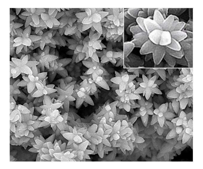
A scanning electron microscope image shows titanium dioxide "nanoflower" structures on the superomniphobic device surface. Credit: Sanli Movafaghi/Colorado State University
