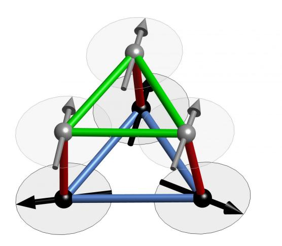
A section from the crystal lattice of Calcium-chromium oxide showing how the spins are subject to conflicting demands. In this ball-and-stick model, the green and red sticks connecting the atoms (grey and black balls) represent ferromagnetic interactions while the blue sticks represent anti-ferromagnetic interactions. Credit: HZB
