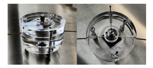
Test set-up for the silicon battery: the battery itself is only the size of a button cell and is located in the hollow cylinder in the middle of the acrylic glass casing. The thin channels that pass through the housing control the supply and outlet of the electrolyte fluid. Credit: Forschungszentrum Jülich
