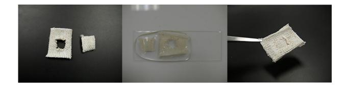
SRT coated fabric self-heals. From left, fabric with hole, wet fabric and patch in a drop of water, self-healed fabric. Credit: Demirel Lab / Penn State
