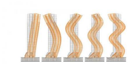
Models of mode shapes for building motion. Credit: Image courtesy of M. Kohler/Caltech
