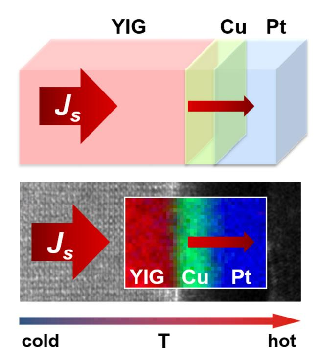
Thermally excited spin waves carry a spin current from the ferromagnet (YIG in this case) into the metal layer. Depending on the YIG thickness and the interface condition the amplitude of the spin current as well as transmission properties change. Credit: Joel Cramer, JGU
