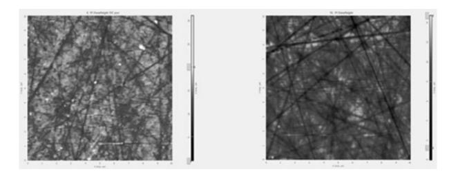
AFM of the surface of 6H-SiC. On the left: surface before planarization; on the right: after 15 minutes of radiation by ion-cluster beam. Credit: National Research Nuclear University
