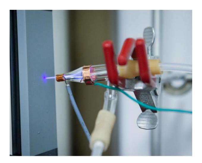
he plasma jet printer consists of a glass nozzle with two copper electrodes connected to a power supply. Credit: Universities Space Research Association at NASA Ames Research Center
