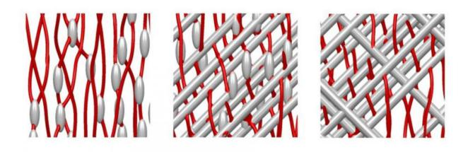
In a new study, researchers at Argonne have developed a rational approach to optimizing the arrangement of defects in commercial high-temperature superconducting wires to enhance their current-carrying capacity. This snapshot of a simulation shows the defects in the material, here in gray, and pinning vortices, in red. The pinning enhances the superconducting behavior of the material at high magnetic fields. Credit: Argonne National Laboratory
