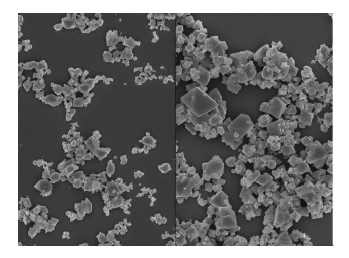
Low gravity was found to increase crystal size. On the left is the crystal formation of a Metal-Organic Framework grown at normal gravity. On the right is the same MOF grown at low gravity generated by skydiving. Credit: Dr Joseph Richardson et. al.
