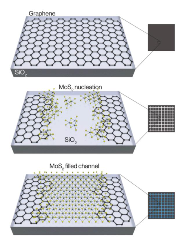
This schematic shows the chemical assembly of two-dimensional crystals. Graphene is first etched into channels and the TMDC molybdenum disulfide (MoS2) begins to nucleate around the edges and within the channel. On the
