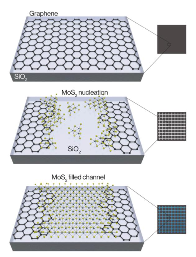
This schematic shows the chemical assembly of two-dimensional crystals. Graphene is first etched into channels and the TMDC molybdenum disulfide (MoS2) begins to nucleate around the edges and within the channel. On the
