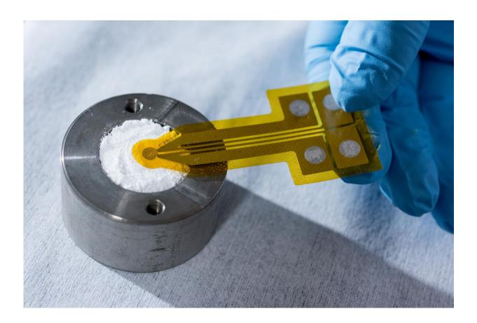
A thermal probe tests heat conductance in a sample of silicon dioxide nanoparticles. The material could potentially conduct heat at an efficiency higher than that of conventional materials. Credit: Rob Felt, Georgia Tech
