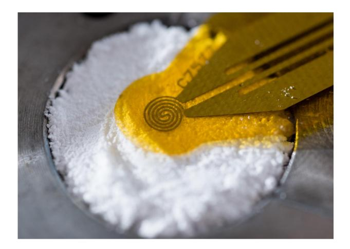
A thermal probe tests heat conductance in a sample of silicon dioxide nanoparticles. The material could potentially conduct heat at an efficiency higher than that of conventional materials. Credit: Rob Felt, Georgia Tech
