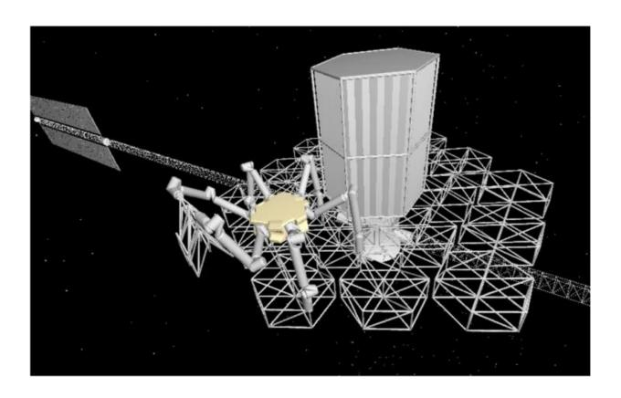
The conceptual CAD rendering of an assembly robot deploying a truss module. Folded truss modules are stored in a cargo housing unit shown docked to the central hub. Credit: doi:10.1117/1.JATIS.2.4.041207
