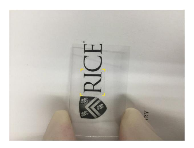
Rivet graphene (outlined in yellow) is nearly as transparent as pure graphene and retains its strength and conductivity even when flexed. The material was created at Rice University. Credit: Tour Group/Rice University
