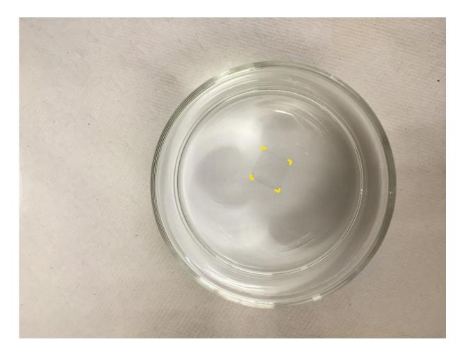
A sheet of rivet graphene (outlined in yellow) floats in water. The enhanced graphene created at Rice University can be transferred from its growth substrate without the need for contaminating polymers. Credit: Tour Group/Rice University
