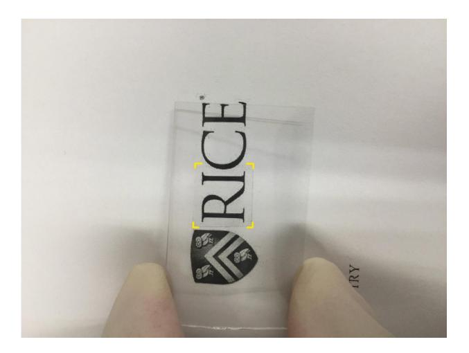
Rivet graphene (outlined in yellow) is nearly as transparent as pure graphene and retains its strength and conductivity even when flexed. The material was created at Rice University. Credit: Tour Group/Rice University
