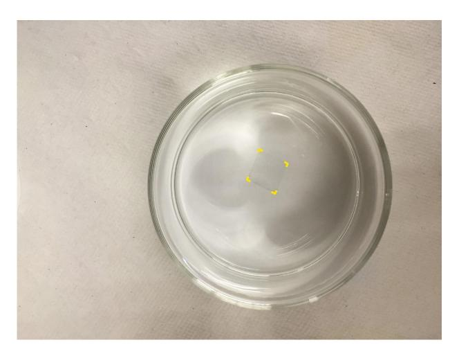
A sheet of rivet graphene (outlined in yellow) floats in water. The enhanced graphene created at Rice University can be transferred from its growth substrate without the need for contaminating polymers. Credit: Tour Group/Rice University
