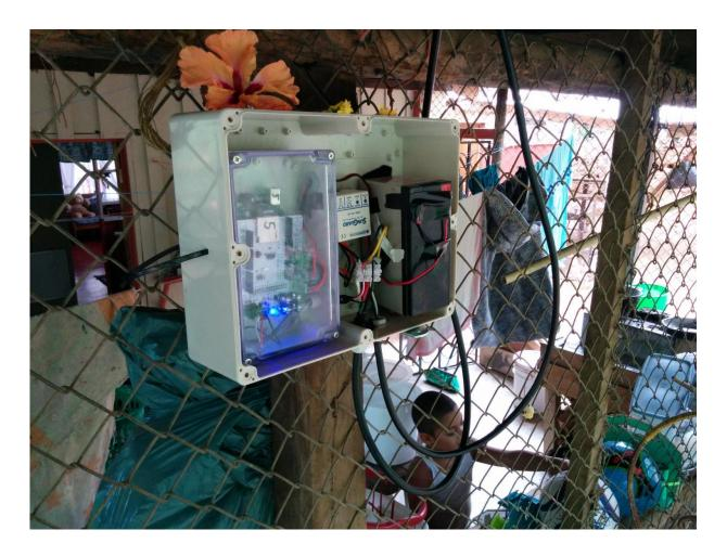
Collaboration with local people living adjacent to streams was important for installing monitoring equipment and providing security for the equipment. The photo shows the automated datalogger at a property along the Caimital River, Costa Rica. Credit: Silja Hund.
