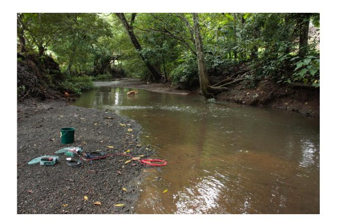
The automated dataloggers can be used for long-term monitoring, as well as for temporary monitoring used to estimate stream flow, as seen in this photo from the Potrero River, Costa Rica. Credit: Silja Hund.
