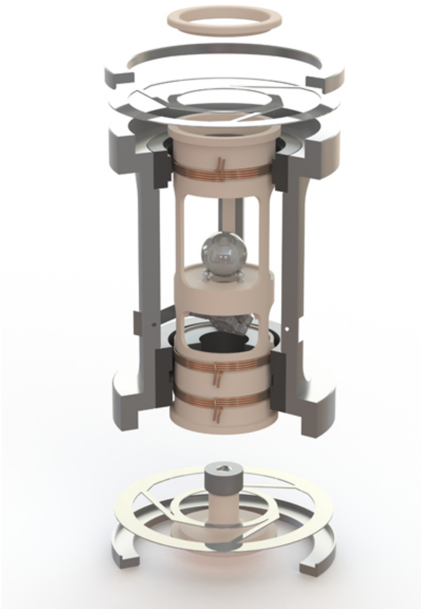
NPL's design for the next-generation of Kibble balances. Credit: National
