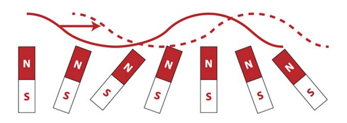
This illustration shows how the magnetic fields of individual atoms, reimagined as bar magnets, change position like tiny compasses when heat or a current is applied to a solid material. The repositioning creates a spin wave, shown by the dotted line. These spin waves are being studied for potential use in microelectronics. Credit: Michael Flatté laboratory.
