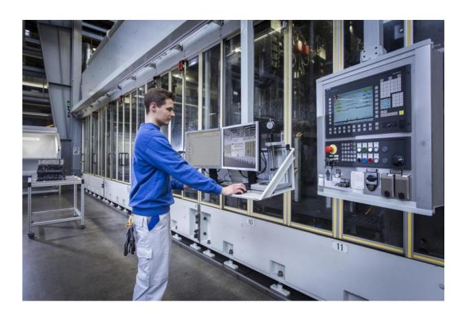
The honing machine at VW's plant in Salzgitter. Experts from the Fraunhofer IFF in Magdeburg have developed a digital assistance system for quality inspection and integrated it in the production process. Credit: Fraunhofer IFF
