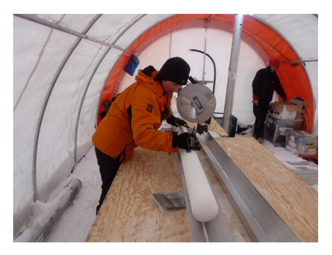
Retrieving and measuring an ice core from the deep field. Credit: British Antarctic Survey
