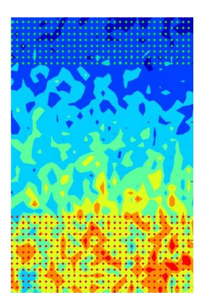
Solidification under sedimentation: The dynamic map illustrates the speed of the particles in the model system. Regions with low speeds are marked in red and orange while those with higher speeds are blue. Red dots show where a solid has already formed. Similar maps were taken during glass formation, but due to the
