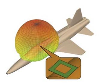
The radiation pattern of patch antenna when installed in actual equipment can now be predicted using a parametric model. Credit: A\*STAR Institute of High Performance Computing
